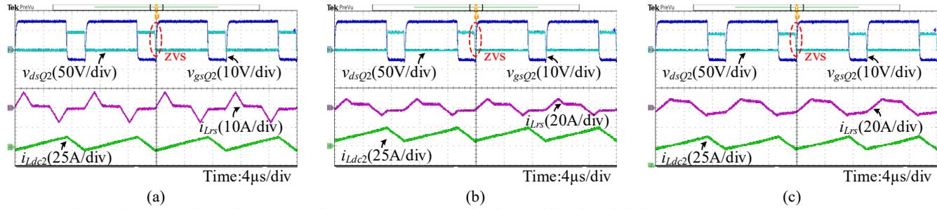
Fig.17. Soft-switching waveforms for  $Q_1$ & $Q_2$  when  $V_L = 12V$ . (a)light load. (b)half load. (c)full load.
