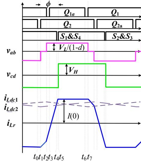
Fig.2. Steady-state waveforms of PPS for CF-DAB in boost mode. (interval A:  $\phi \in [(2d-1)\pi, \pi]$ ).
