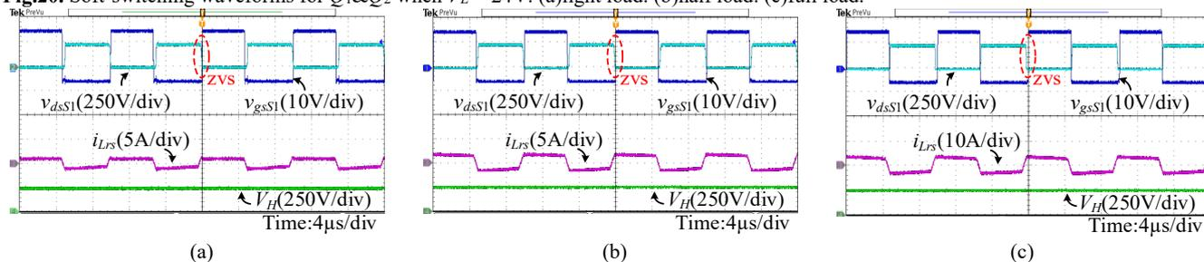
Fig.21. Soft-switching waveforms for  $S_1$  &  $S_2$  &  $S_3$  &  $S_4$  when  $V_L = 24V$ . (a)light load. (b)half load. (c)full load.
