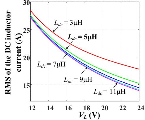
**Fig.9.** RMS currents under different DC inductor values.
