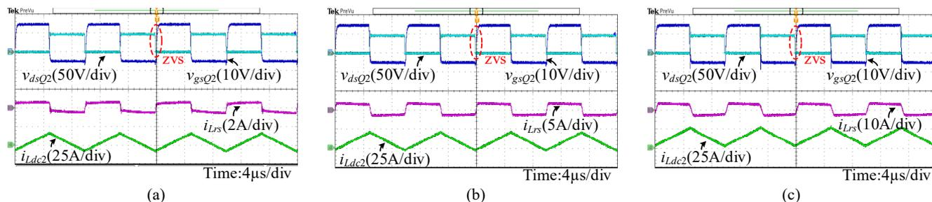
Fig.20. Soft-switching waveforms for  $Q_1$  &  $Q_2$  when  $V_L = 24V$ . (a)light load. (b)half load. (c)full load.
