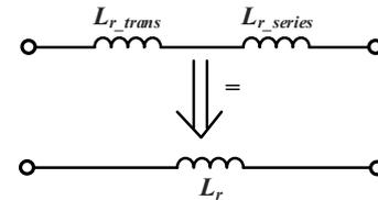
Fig.12. The diagram of leakage inductor.
