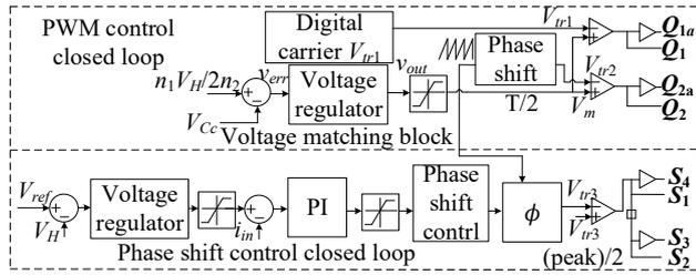
Fig.4. The diagram of the decoupling control.
