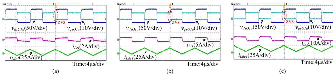
Fig.19. Soft-switching waveforms for  $Q_{1a}$  &  $Q_{2a}$  when  $V_L = 24V$ . (a)light load. (b)half load. (c)full load.
