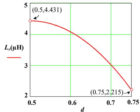
Fig.7. Relation between transmission power to leakage inductance and duty cycle. ( $\phi = 0.5\pi, P_N = 650W$ ).
