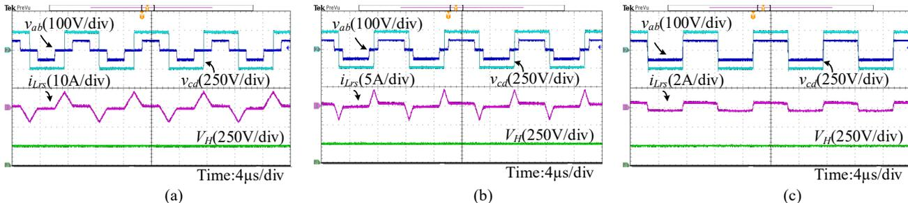
Fig.13. Steady-state waveforms under light load. (a)12V. (b)18V. (c)24V.
