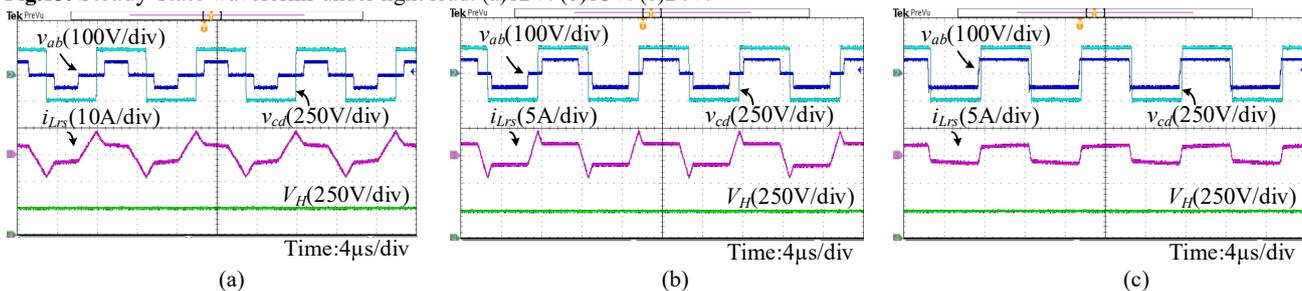
Fig.14. Steady-state waveforms under half load. (a)12V. (b)18V. (c)24V.
