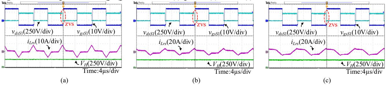
Fig.18. Soft-switching waveforms for  $S_1$ & $S_2$ & $S_3$ & $S_4$  when  $V_L = 12V$ . (a)light load. (b)half load. (c)full load.
