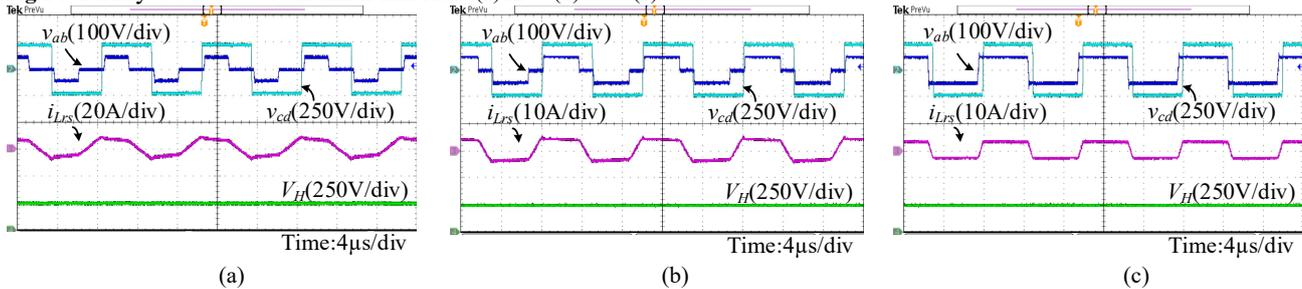
Fig.15. Steady-state waveforms under full load. (a)12V. (b)18V. (c)24V.
