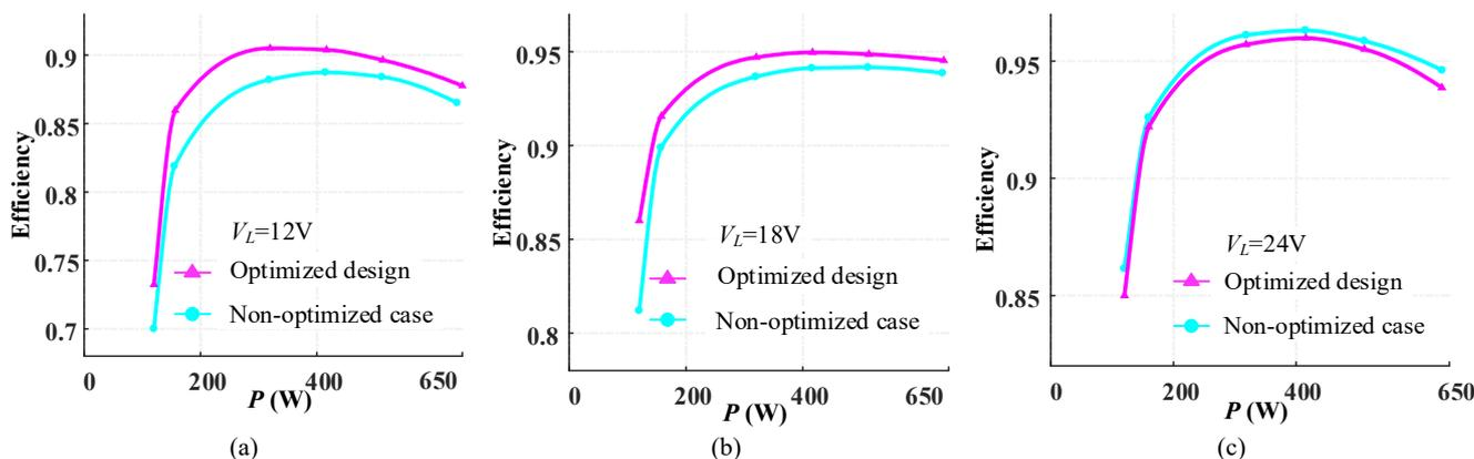
Fig.22. Comparison of efficiency curves between optimized design and non-optimized case of the converter. (a) when  $V_L=12V$ . (b) when  $V_L=18V$ . (c) when  $V_L=24V$ .
