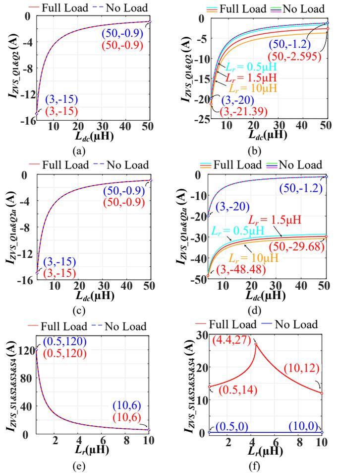
**Fig.6.** Current at switch turn-on. (a)  $Q_1\&Q_2$   $V_L = 12V$ . (b)  $Q_1\&Q_2$  when  $V_L = 24V$ . (c)  $Q_{1a}\&Q_{2a}$   $V_L = 12V$ . (d)  $Q_{1a}\&Q_{2a}$  when  $V_L = 24V$ . (e)  $S_1\&S_2\&S_3\&S_4$  when  $V_L = 12V$ . (f)  $S_1\&S_2\&S_3\&S_4$  when  $V_L = 24V$ . ( $V_L = 12 \sim 24V$ ,  $V_H = 240V$ ,  $P_N = 650W$ ).
