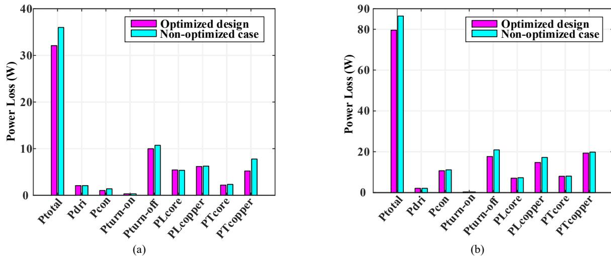
Fig.10. Loss breakdown when  $V_L = 12$  V. (a). at light load ( $P = 120$ W). (b). at full load ( $P = 650$ W).
