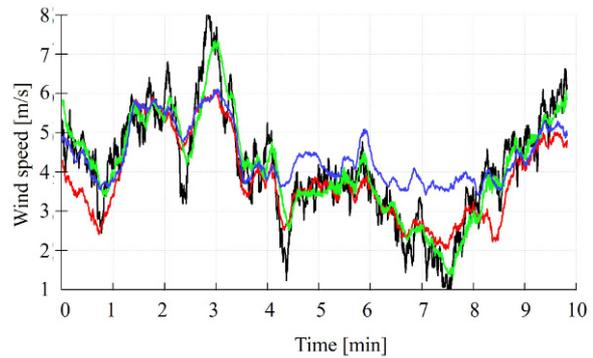
Fig. 1. Simulation results of the nacelle wind, the baseline EWS and two estimated EWSs at 4 m/s mean wind speed.
