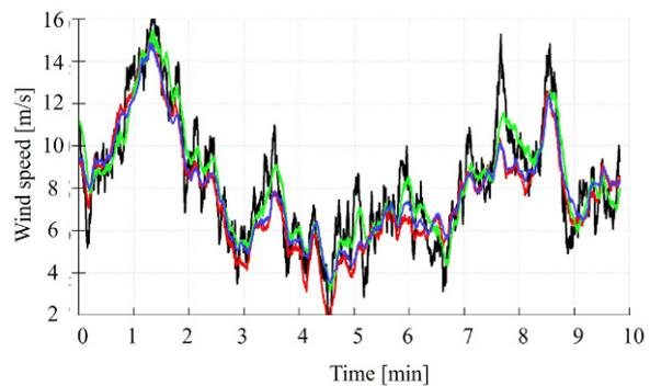
Fig. 2. Simulation results of the nacelle wind, the baseline EWS and two estimated EWSs at 8 m/s mean wind speed.
