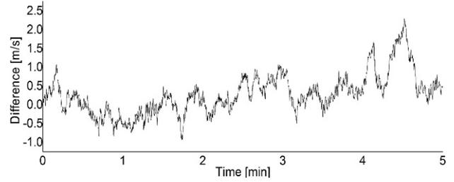
Fig. 6. Difference between the baseline EWS and the EKF-based estimated EWS at 8 m/s mean wind speed.
