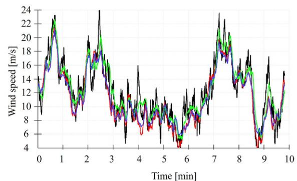
Fig. 3. Simulation results of the nacelle wind, the baseline EWS and two estimated EWSs at 12 m/s mean wind speed.
