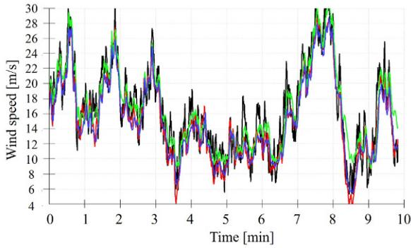
Fig. 4. Simulation results of the nacelle wind, the baseline EWS and the estimated Kalman filter-based WES at 16 m/s mean wind speed.
