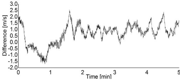
Fig. 5. Difference between the nacelle wind speed and the baseline EWS at 8 m/s mean wind speed.
