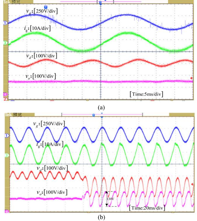
Fig. 5. Experimental waveforms of grid voltage  $v_g$ , grid current  $i_g$ , capacitor voltage  $v_d$ , and load voltage  $v_o$ . (a) Steady-state experimental waveforms. (b) Dynamic experimental waveforms.
