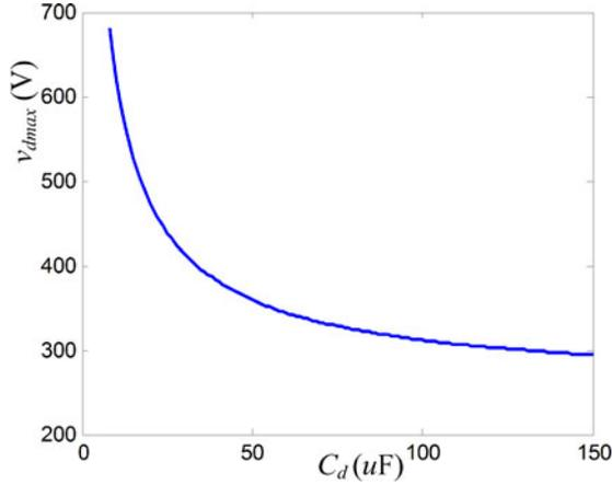
Fig. 3. Plot of voltage stress against the capacitance.
