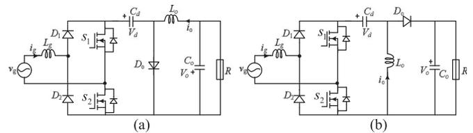
Fig. 1. Bridgeless PFC rectifier based on (a) Cuk [8] and (b) Sepic circuits [10].
