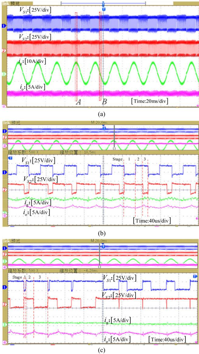
Fig. 6. Experimental waveforms of gate-emitter voltages, grid current  $i_g$ , and inductor current  $i_o$ . (a) Waveforms of  $V_{s1}$ ,  $V_{s2}$ ,  $i_g$ , and  $i_o$ . (b) Zoom-in waveforms of point A. (c) Zoom-in waveforms of point B.
