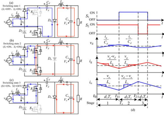
Fig. 2. Switching states of bridgeless Cuk PFC rectifier in the positive half-line cycle and theoretical waveforms. (a) State 1. (b) State 2. (c) State 3. (d) Theoretical waveforms.
