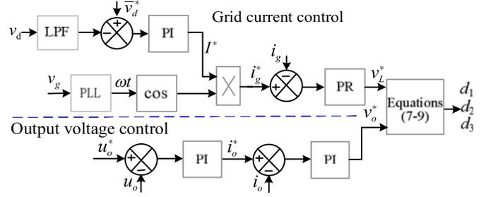
Fig. 4. Block diagram of the control scheme.
